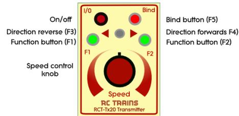
**On/off switch** - *Illuminated push-push switch*. The LED shines steadily during normal operation; it flashes once a second during the binding process and it flashes erratically when the battery is depleted.
