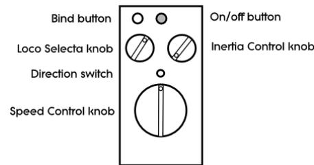
**On/off switch** - *Illuminated push-push switch*. The LED shines steadily during normal operation; it flashes once a second during the binding process; it flickers rapidly while inertia control is in operation (see below) and it flashes erratically when the battery is depleted. It also flashes to guide and confirm **additional functions** (see below).
